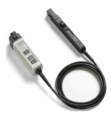
TCP0030A is a high-performance, easy-to-use AC/DC current probe designed for use and direct connection to oscilloscopes with the TekVPI<sup>™</sup> probe interface. This AC/DC current measurement probe provides greater than 120 MHz of bandwidth with selectable 5 A and 30 A measurement ranges. It also provides exceptional low-current measurement capability and accuracy to current levels as low as 1 mA, important for meeting today's challenging current measurement needs.
